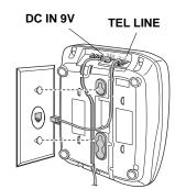
4. For a wall plate, plug the modular cord's other end into the wall plate jack, then align the base's keyhole slots with the wall plate studs and slide the base downward to secure it. For direct wall mounting, align the base's keyhole slots with the mounting screws and slide the base downward to secure it.
